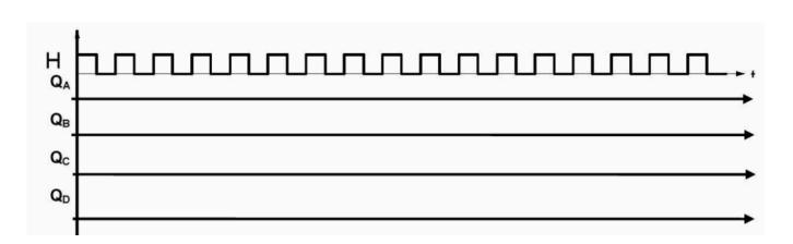
4- Wire the implementation from the previous figure to achieve an asynchronous modulo-14 counter
