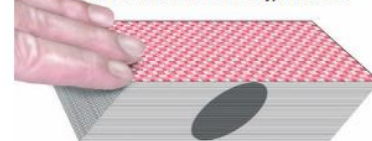
FIGURE 10.3 Shearing and the resulting deformation (strain) An ordinary deck of playing cards with a circle embossed on its side illustrates shearing and the resulting strain.
