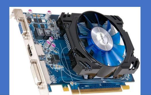
The graphics card, although essential for certain purposes, is listed last in this description because it can be replaced by an integrated chipset (a set of circuits) directly on the motherboard. However, for some applications, especially gaming, it is indispensable. By handling the display management, it relieves the processor of this task, processes information on its own, and uses its dedicated memory, which can significantly improve graphics performance.
