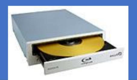
The optical drive, or burner, is attached to the case and is inserted into an open slot on the front of the PC. This allows for the opening of the tray that receives the optical disc, more commonly referred to as a CD (Compact Disc) or DVD (Digital Versatile Disc). It is connected to the motherboard via a flat cable (ribbon cable).
