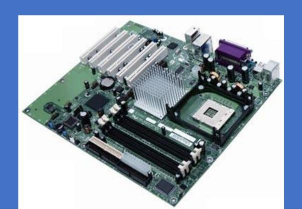
The Random Access Memory (RAM) is used by the processor to temporarily store data during their processing. One of the advantages of the memory used in computers is indeed its fast access speed.
