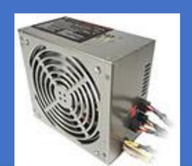
Of course, even if you have all the components listed below, nothing will work without the electrical current supplied by the power supply. It transforms and provides the energy required for the valuable motherboard, to which a good number of elements are connected. However, the power supply is also directly connected to certain components such as the DVD reader/writer or the hard drive, for example.
