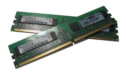
Another characteristic of RAM is that it is temporary; once the operation is completed, the data is not retained and is permanently lost when the computer is turned off.
