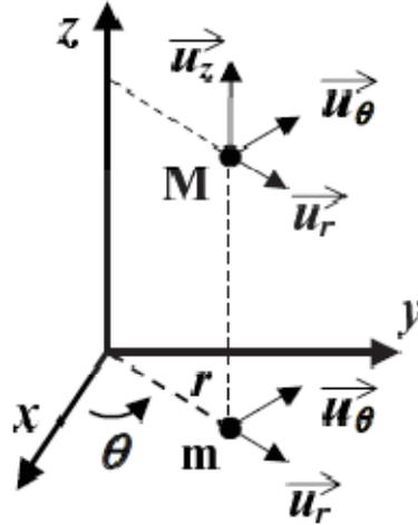
$$\overrightarrow{\text{grad}}V = \frac{\partial V}{\partial r} \vec{u}_r + \frac{1}{r} \frac{\partial V}{\partial \theta} \vec{u}_\theta + \frac{\partial V}{\partial z} \vec{u}_z$$
