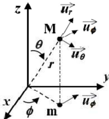
$$\overrightarrow{\text{grad}}V = \frac{\partial V}{\partial r} \vec{u}_r + \frac{1}{r} \frac{\partial V}{\partial \theta} \vec{u}_\theta + \frac{1}{r \sin \theta} \frac{\partial V}{\partial \phi} \vec{u}_\phi$$
