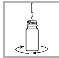
3. Add one drop of Hardness 2 Indicator to the mixing bottle. Swirl to mix.
