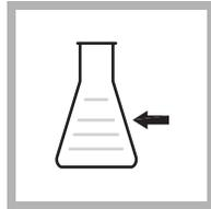
1. Fill the flask to the 100-mL mark with sample.
