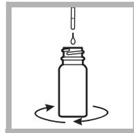
2. Add three drops of Buffer Solution, Hardness 1 to the mixing bottle. Swirl to mix.
