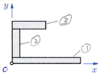
$$\begin{aligned} x_G &= \frac{22.5(4 \cdot 45) + 2.5(5 \cdot 20) + 10(6 \cdot 20)}{4 \cdot 45 + 5 \cdot 20 + 6 \cdot 20} \\ &= \frac{5500}{400} = \underline{\underline{13.75 \text{ mm}}}, \end{aligned}$$
