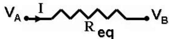
$$V = V_A - V_B = (V_A - V_1) + (V_1 - V_2) + (V_2 - V_B)$$
