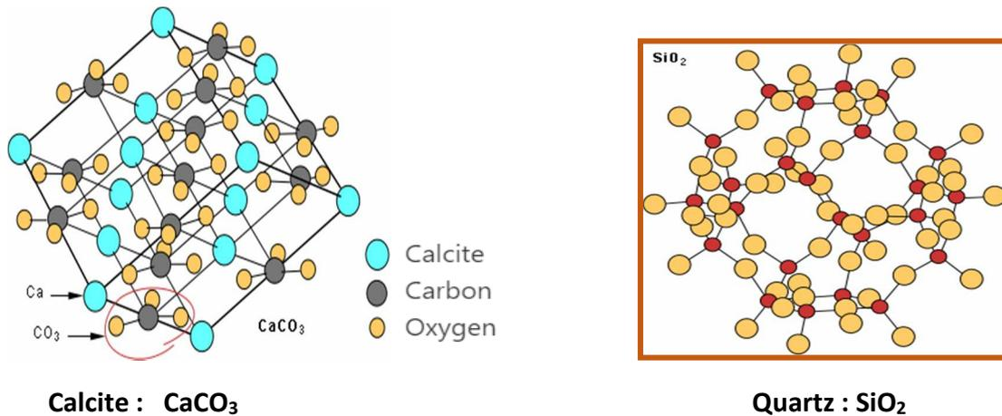
Fig. 3 .The elementary crystal lattice
