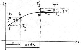
Let T be the tension of the string, under equilibrium conditions the string is rectilinear. Assume that we slowly move the string a small amount. We consider a segment AB of the string of length dx which has been displaced by a distance  $\xi$  from its equilibrium position.
