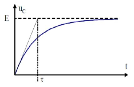
The charge of the capacitor is not instantaneous, it is a transient phenomenon.
