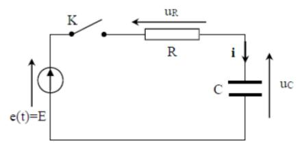
At time t = 0, we close the switch K (the capacitor is initially discharged). The capacitor will gradually charge until a voltage opposite to the emf E is established at its terminals.
