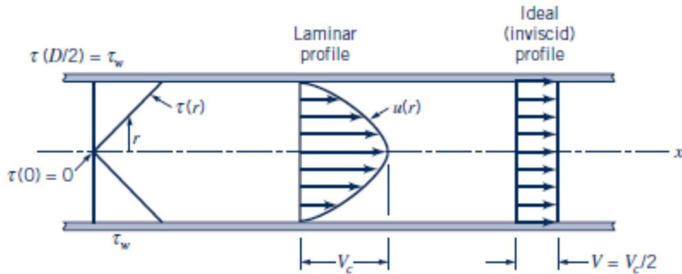
We know that the friction stress in a Newtonian fluid is proportional to the speed gradient:
