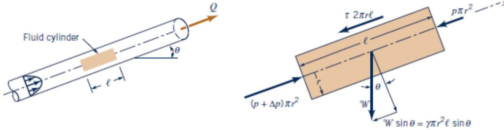
The forces applied to the cylindrical element are:
